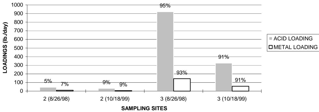
In tributary 3, site 3B was producing 92% of the acidity loading and 93% of the metal loading. Based on available water quality data, site 3B is the largest contributor of AMD in the Goose Run sub-watershed followed by site 2F and a host of low-priority sites. These sources are described in more detail in the following sections.
